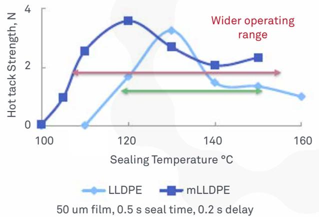
**Figure 3. Hot tack strength test of LLDPE and mLLDPE polymers**
