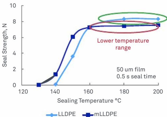
**Figure 2. Sealing curves for LLDPE and mLLDPE using a hot jaw sealer**
