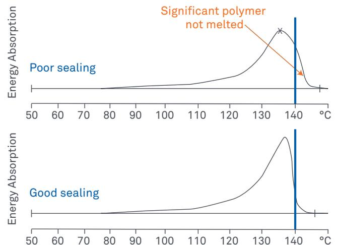
**Figure 8.** DSC curves show the amount of energy being used to melt the polymer over a temperature range. At any given temperature, a higher energy level indicates that more of the polymer is melting at that temperature.
