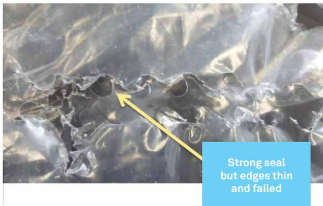
**Figure 6.** Thin and torn edges adjacent to the strong seal indicate excessive temperature in sealing, particularly in areas where little powder was observed.
