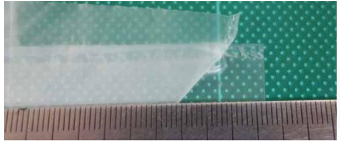
**Figure 7.** Seal failure of a HDPE bag
