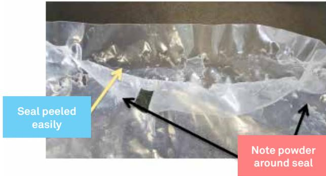
**Figure 5.** Seal failure in many seals due to peeling, particularly where powder was observed.
